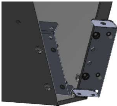
Installation of connector inside the curtain
